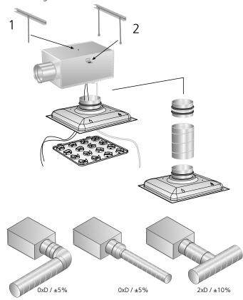
Figure 1. Installation 1 = Pop-nuts 2 = Mounting brackets
