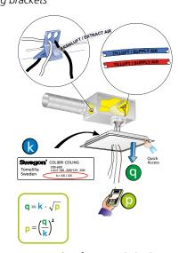
Figure 2. Measurement tubes for commissioning.
