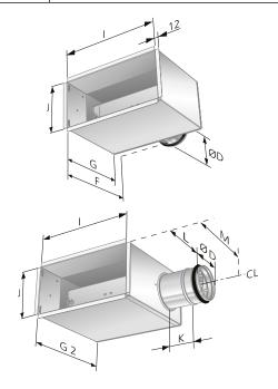
Figure 2. ALV commissioning box. B = Rear connection, K = Connection on short side, CL = Centre line.
