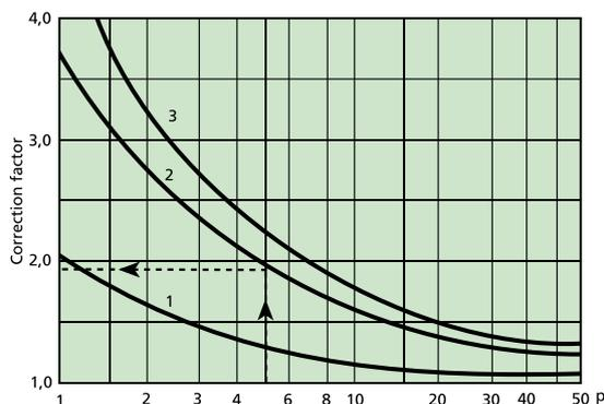
Curve 1: Plenum-Duct, Curve 2: Duct-Plenum, Curve 3; Plenum-Plenum
